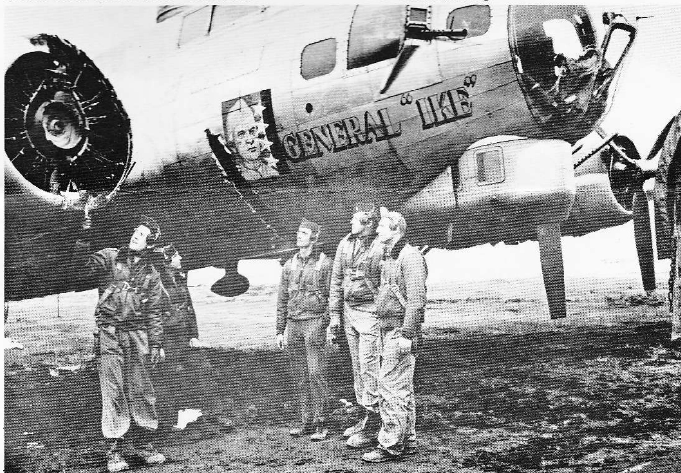
Examining damage caused by a lost prop following a combat mission in "General Ike."
