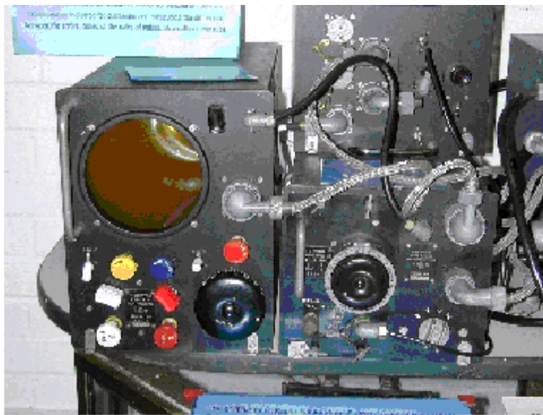
The British GEE box is the unit with the cathode ray tube (above left). Basically, the GEE box is an oscilloscope, an electronic instrument that produces an instantaneous visual display or trace of electron motion on the screen of a cathode ray tube. Only the unit with the cathode ray tube sat on the navigator's table. The other two support units were mounted in other parts of the aircraft. The GEE box at the left is displayed at the Pitstone Navigation Museum in Pitstone, England. It should be noted that this unit does not have a daylight visor used by 8th Air Force navigators. The RAF bombers always flew at night and the light shields were not required.
